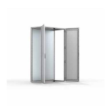
The mild steel double door combinable floor standing enclosure range, MCD, is ideal for installation in confined spaces where a single door, when opened, would take up too much space in front of the enclosure. The doors' loading capacity also increases as it is divided over two doors. With a IP 55 protection degree, components inside the enclosure are well protected and makes it well suited for many different applications.
